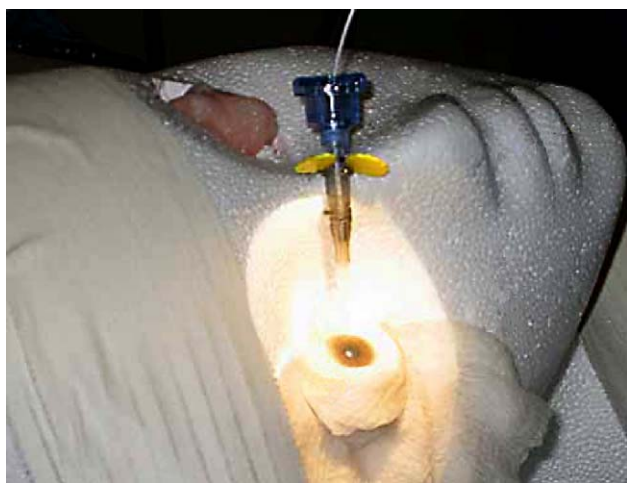
Figure 1. Setup of the vitreous pressure transducer. The transducer is located in the vitreous cavity at the tip of the catheter wire.
